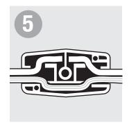
Place uncut ribbed cord in open channel of hollow half of switch. Tuck two cut ends of non-ribbed cord into top portion.
