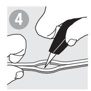
Cleanly cut non-ribbed wire in half at center of slit. Do not strip wire.
